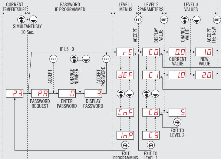
**REMARK:** If no key is pressed for 25 seconds in either of the previous steps, the controller will automatically return to the CURRENT TEMPERATURE display status without modifying any of the parameters values.
